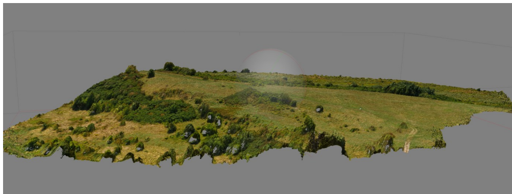
FIG. 4. Fragment of a dense point cloud of the open area (about 5 million points). The illustration clearly shows blank spaces.
