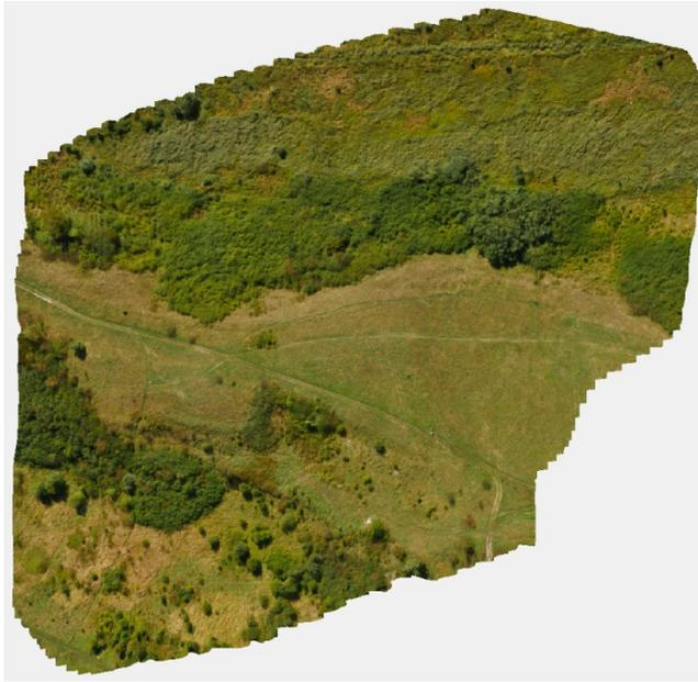
FIG. 6. Fragment of an orthophoto map generated from stitched photos.
