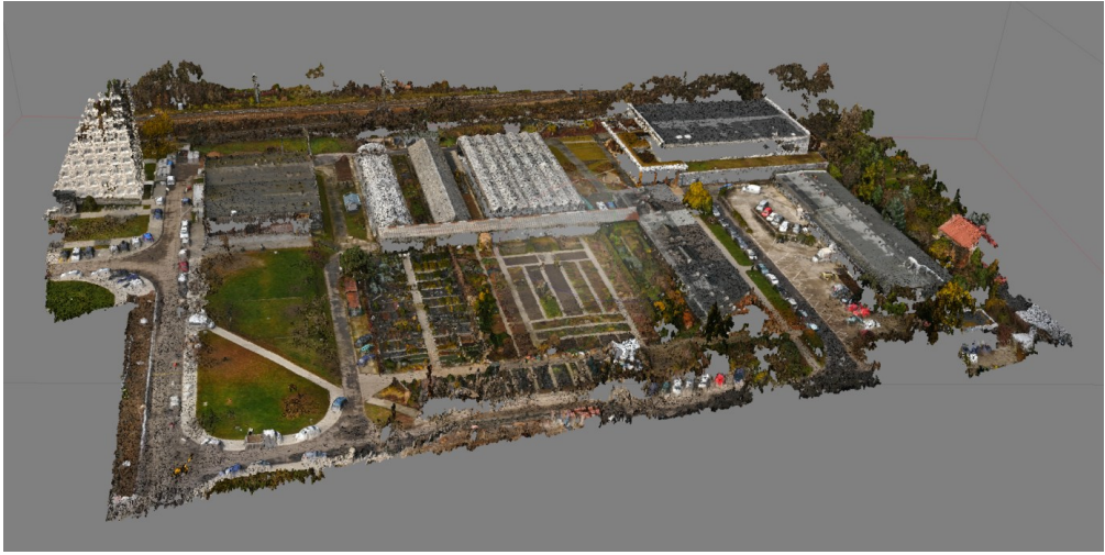
FIG. 2. Example of a dense point cloud containing over 53 million points.
