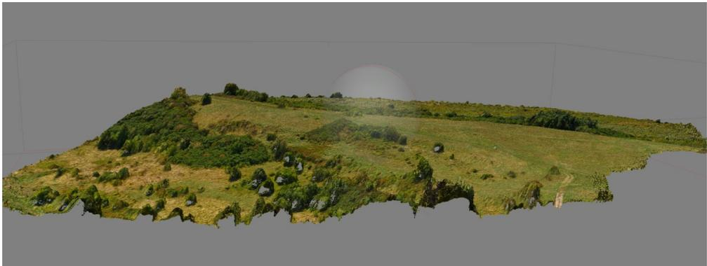
FIG. 4. Fragment of a dense point cloud of the open area (about 5 million points).
