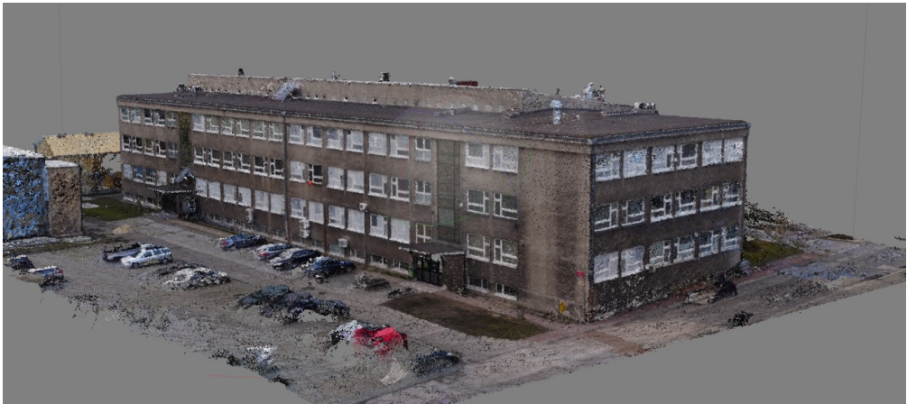
FIG. 9. Fragment of a dense point cloud of an architectural object (about 7 million points).
