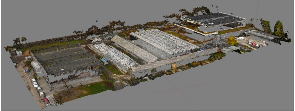
FIG. 7. Fragment of a dense point cloud of the built-up area (about 23 million points).
