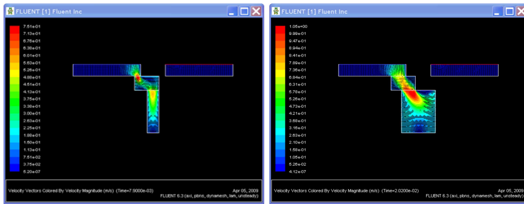
Fig. 8. Oil velocity vector distribution at the moment of connecting the working chamber with the low pressure port.
