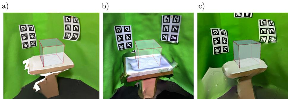
FIG. 2. Views from Unity showing the placement of the virtual cube in the mapped space for the AR platforms: a) Vuforia, b) Immersal, c) MultiSet.
