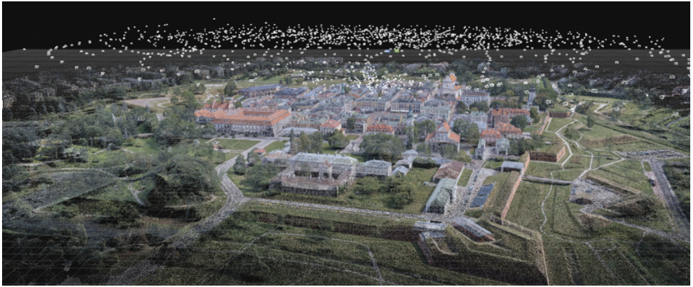
FIG. 3. Photogrammetry-derived point cloud and camera network (all image positions) generated in RealityCapture [33].
