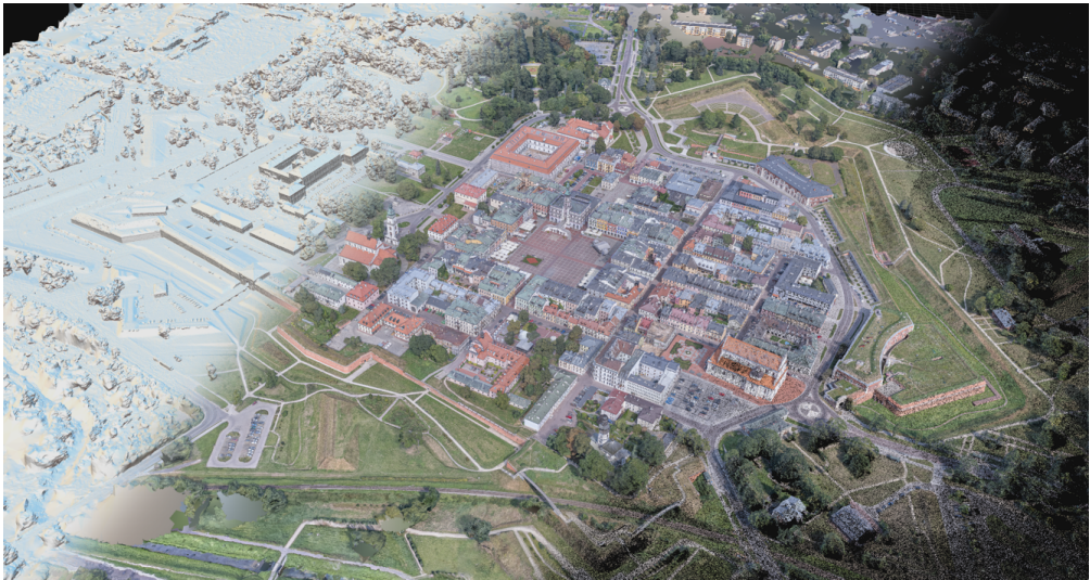
FIG. 5. Integration of TLS point cloud and UAV photogrammetric model for Zamość Old Town (left: raw 3D model, centre: textured 3D model, right: point cloud) visualised in RealityCapture.
