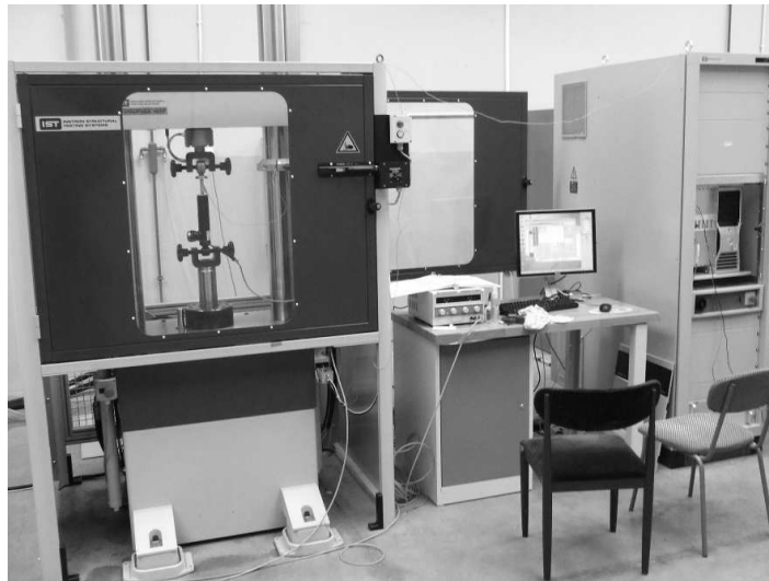
Fig. 16. A servo-hydraulic test rig used in experimental investigations.
