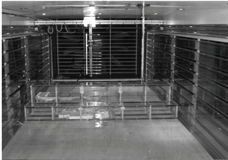
Fig. 1. The arrangements of models in measurements space in the wind tunnel
