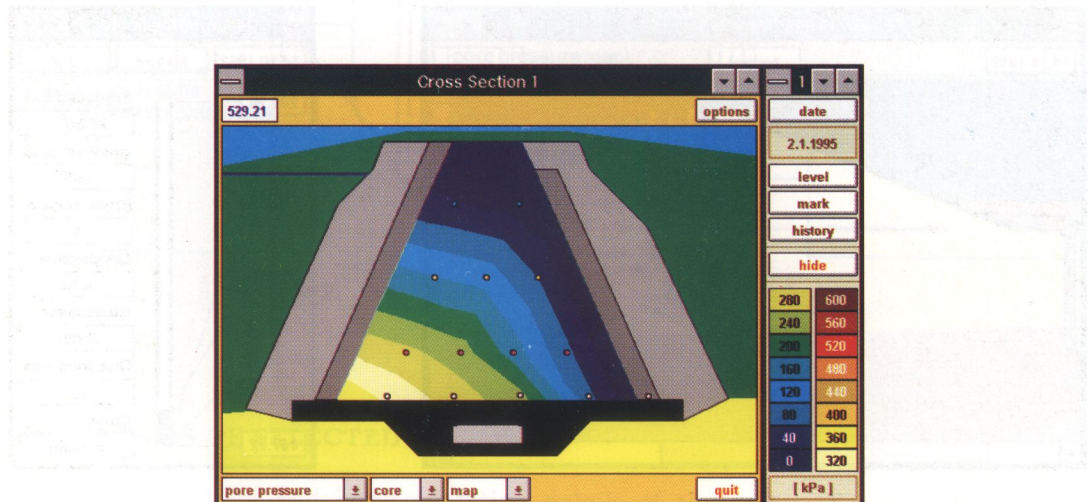
Fig. V. Cross section view with accompanying options window (CZORSZTYN dam)
