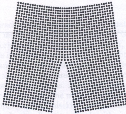
Fig. 10. Picture of the cracked three-point bend beam part (A)
